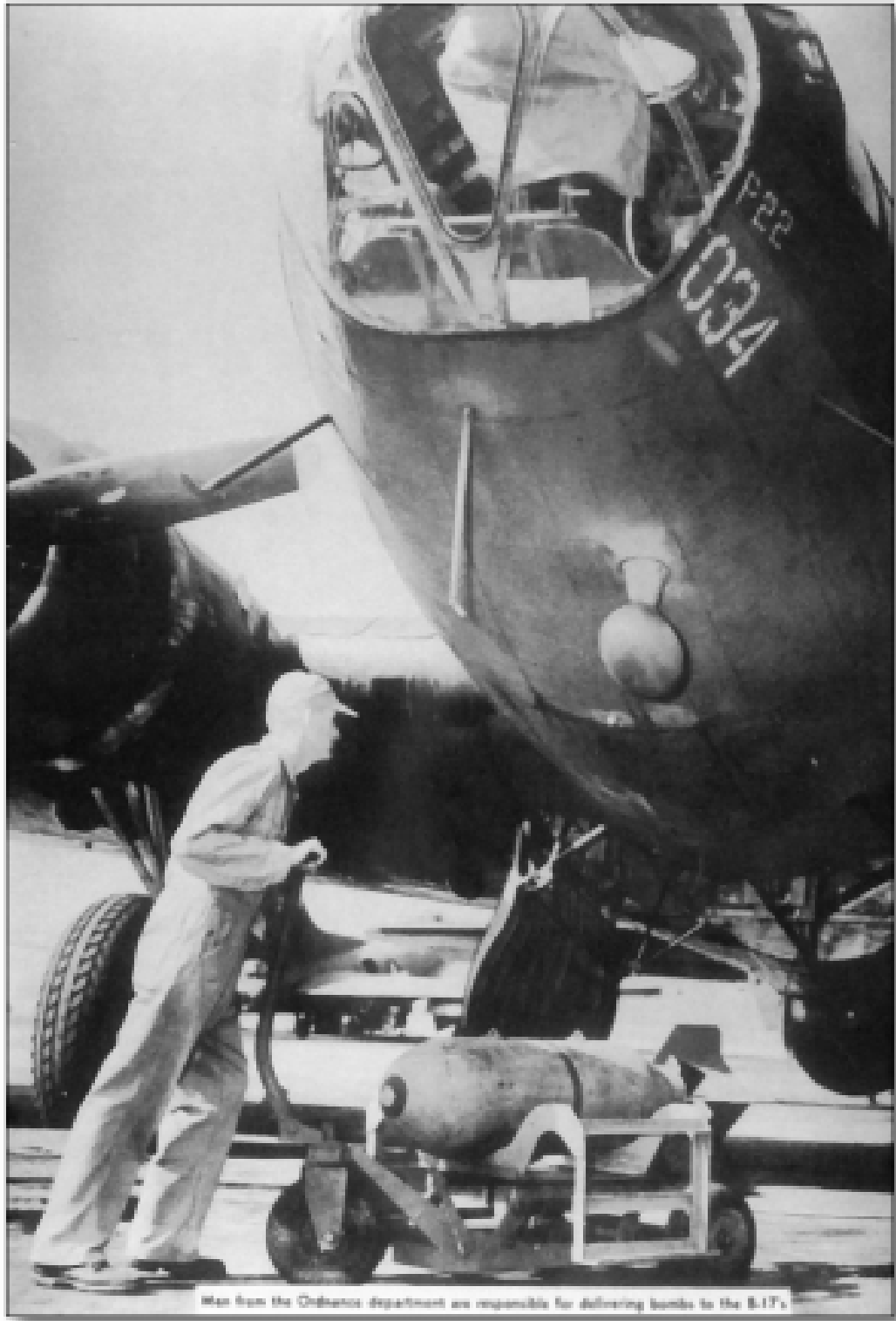
An ordnance man loading a bomb on a B-17 for a practice mission.
